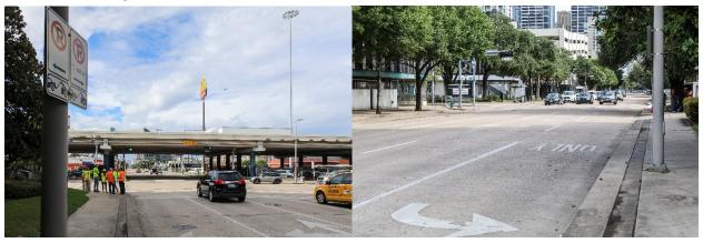
Figure 20: Dual left turn lane configuration.
