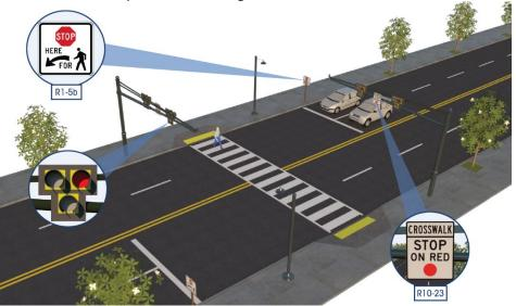
Figure 16: Pedestrian Hybrid Beacon (PHB).
