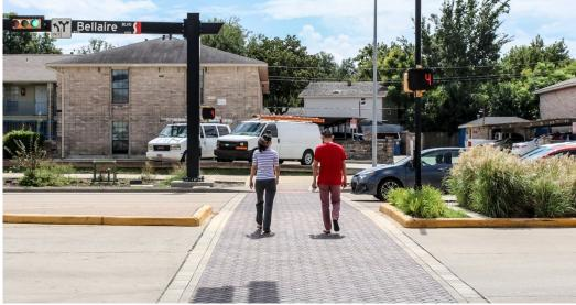
Figure 34: Median pushbutton and crossing timing to cross half way per cycle.
