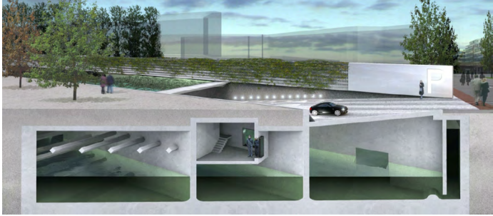
Water detention in underground parking. Images credit: Municipality Rotterdam Above: Detention in roof construction of Kruisplein garage Below: Detention in left-over spaces in parking garage museum square
