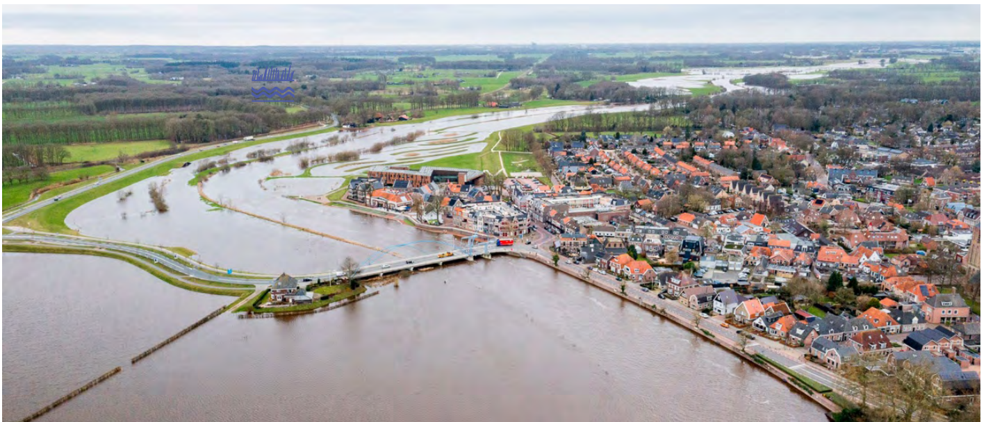
Flooded park with meandering water trenches next to Dalfsen, NL during winter 2022. Most of the time, the park is dry and used for recreation. Image credit: Thomas Klomp
