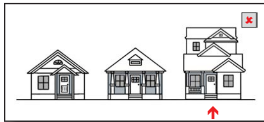
Incompatible addition; visually dominates original building
