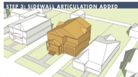
STEP 3: SIDEWALL ARTICULATION ADDED An offset of the sidewall facade further defines the proportions of the structure. This tool can reduce the perception of mass from the sideyard realm for neighboring properties.
