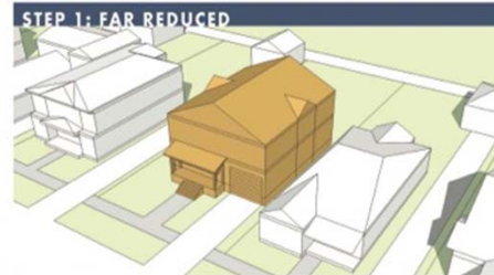
STEP 1: FAR REDUCED Floor-Area-Ratio (FAR) is the ratio between floor area and the lot size. A reduction in the FAR limits the amount of floor space in the residence, but does not address other massing regulations.
