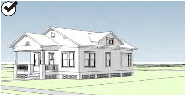
3. Dormer has been added.
