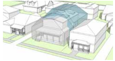
This envelope slopes in from the side property lines, moving taller portions of the mass away from neighbors, reducing the “looming” effect.
