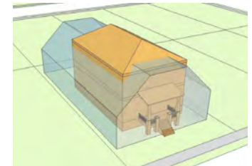
Building exceeds maximum building envelope
