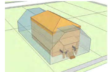
Building exceeds maximum building envelope
