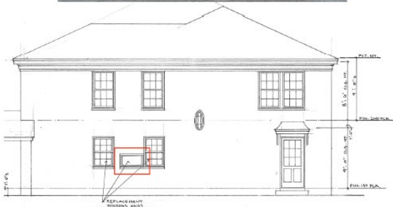
G1 - REPLACEMENT: Window only to be removed – no replacement.
