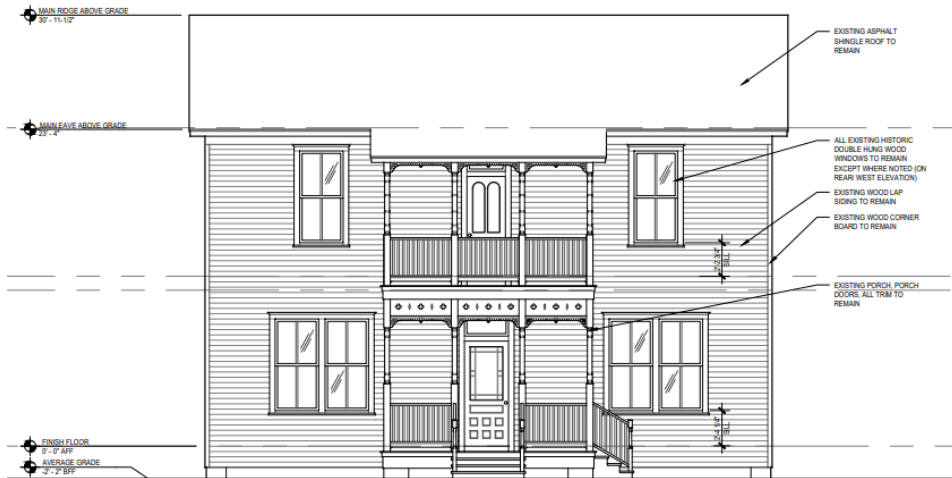
03 EXISTING EAST ELEVATION (FRONT) SCALE: 1/4" = 1'-0"
