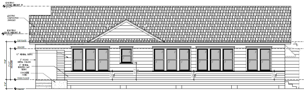
EXISTING HOUSE SOUTH ELEVATION Scale: 1/4" = 1'-0"
