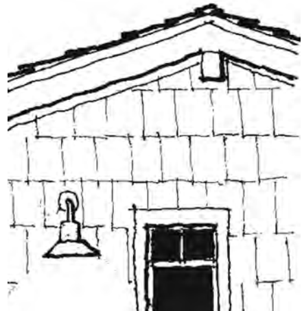
Where possible, use hoods over lightbulbs to direct light downward, which minimizes light pollution.
