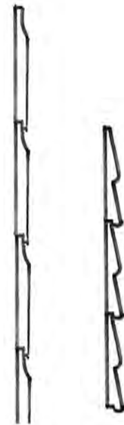
Typical siding profiles in the Heights: (left) 105 and (right) 117
