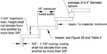
Figure 29. Tread Connection Requirements
