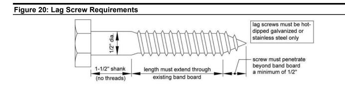
Lag screw installation requirements: Each lag screw shall have pilot holes drilled as follows: 1) Drill a  $\frac{1}{2}$ " diameter hole in the ledger board, 2) Drill a  $\frac{5}{16}$ " diameter hole into the band board of the existing house. DO NOT DRILL A  $\frac{1}{2}$ " DIAMETER HOLE INTO THE BAND BOARD.
