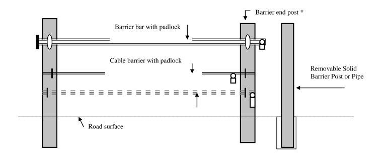
\*An approved "9-1-1" Box <u>shall</u> be provided, on the non-movable barrier post at the lock end of the barrier, containing the key for the lock or a release mechanism to open the barrier. (See Appendix F for description of "9-1-1" Box.)
