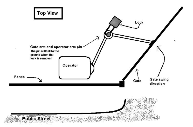
**Note:** When the operator and the gate arms are activated in the normal mode or in the "Fail-safe" mode, the gate shall open such that the <u>full required width</u> of the street, drive or access road will be maintained and the full required width available for emergency use.
