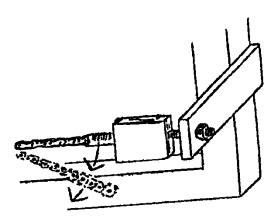
In this illustration the firefighter or other emergency responder unlocks the Falcon Lock located on the "9-1-1" Box. He will pull the handle on the cable that causes the gate operator chain to be released as shown in the lower drawing.
