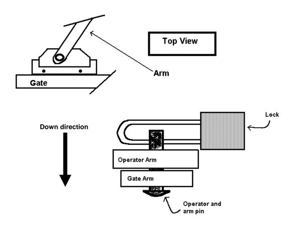
When a pin is used in a "Fail-safe" assembly and the lock is removed, the pin shall be installed such that it will readily fall toward the ground.
